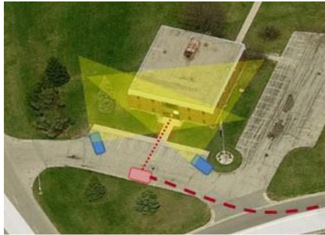
Example of a Protected Entry Corridor
